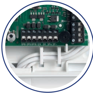
Expander Plus Housing “The optional larger expander box is great for installations with lots of wiring. The cable management hooks help keep it neat.”
