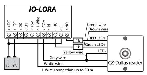
The output xOUT must be set to the "System State" type. Security alarm is on - the iButton reader light is red. The security alarm is off - the iButton reader light is green.
