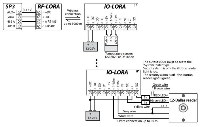
Note: An *RF-LORA* transceiver must be connected to the "*FLEXi*" *SP3* control panel and then up to 8 pcs. can be connected *iO-LORA* wireless expanders.
