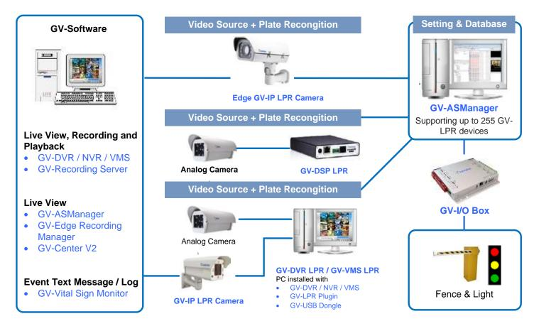
Note: Edge GV-IP LPR Camera includes GV-LPR2811-DL / GV-LPR2800-DL / GV-LPR1200.
